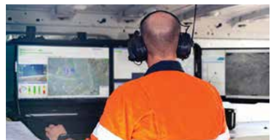
The pilot of the fixed wing drone sits in the back of a van flying the drone using realtime video from the drone and satellite maps to track his position. The drone requires at least two people to operate – the pilot and a ground crew.
