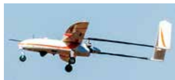
A fixed wing drone take off at the start of the Gregory Park Exhibition. Flown by Insitu Pacific. Insitu is a global company. The drone pictured weighs 20kg and can cruise up to 16km at an altitude of 5000ft for 3.5 hours before needing to refuel. It is required to be manned continually by a certified pilot (as pictured at right).
