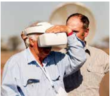
Tony O'Brian tries on the DJI Drone First Person View goggles. Using head movements, the goggles move the drones camera and show the user what the drone can see.
